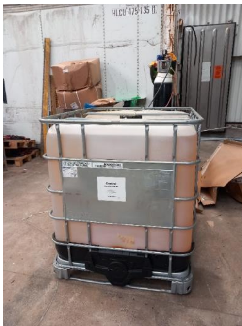
Photo 28. Intermediate Bulk Container (IBC) of hydraulic oil located in Building 55.
